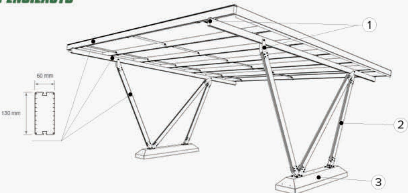
**1 STANDARD COLOUR OF THE POWDER COATING OF THE ALUMINIUM CAPS AND CATAFORESIS TREATED STEEL PLATES**
