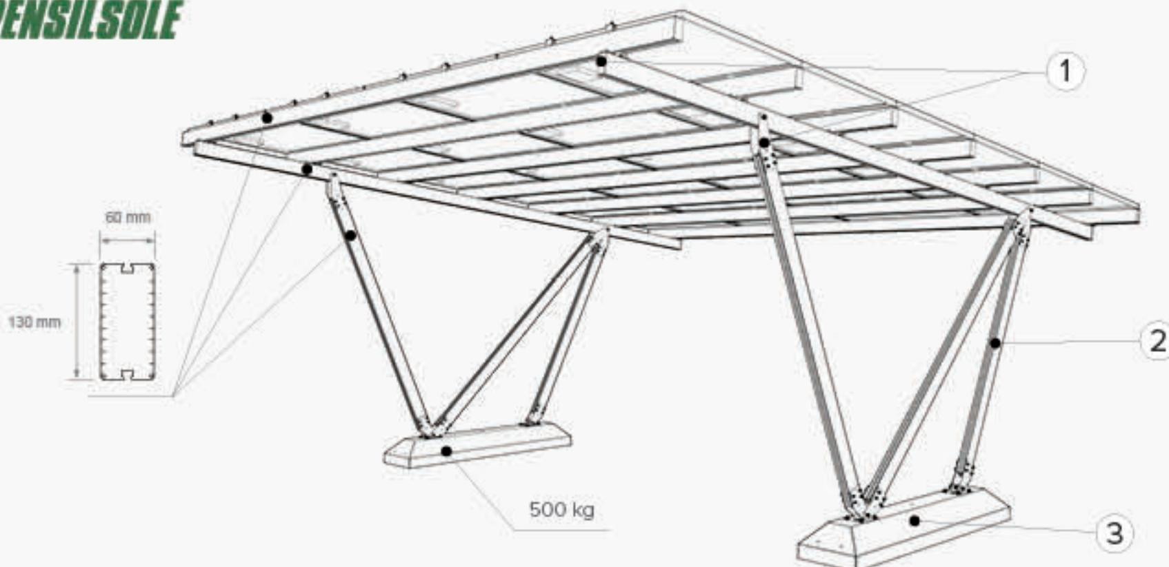
**1** STANDARD COLOUR OF THE POWDER COATING OF THE ALUMINIUM CAPS AND CATAPHORESIS TREATED STEEL PLATES
